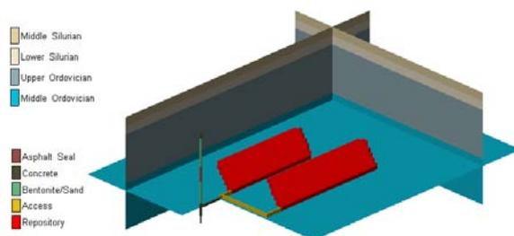
Figure 3. Model discretization showing repository panels, access tunnels, and combined shaft.
