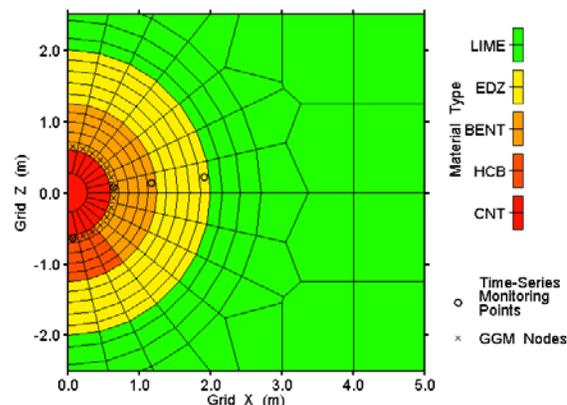
Figure 10. Discretization in container plane.
